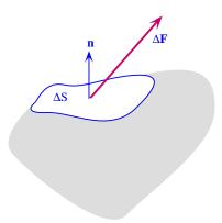
Since we this force is clearly effected by the magnitude  $\Delta S$ , we use instead the force per unit area (the *pressure*) given by
