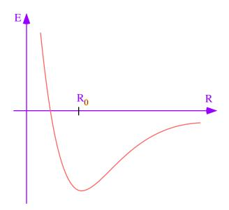
reveals that there is a radius at which the energy is minimum---that is to say, a radius  $R_0$  where the force  $F = -\partial E/\partial R$  is zero and the star is in mechanical equilibrium. A rough calculation of  $R_0$  gives:
